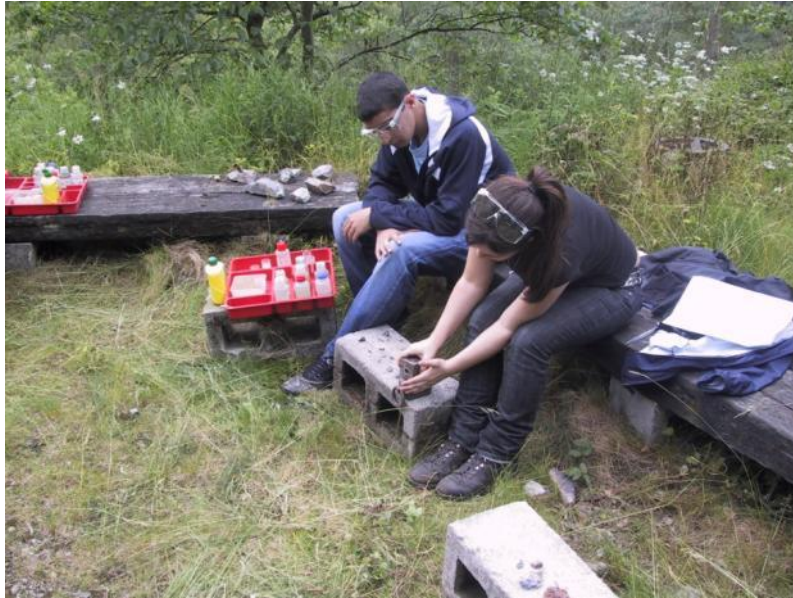
Crushing mineral samples prior to chemical analysis
