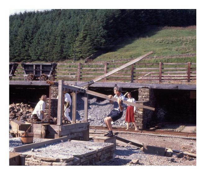
A full-sized jig in use. The jig is made of wood, with a mesh base and is worked up and down in water by a boy pulling on a long handle. Jigs like this were used at Ecton to separate the copper ore from the waste.
